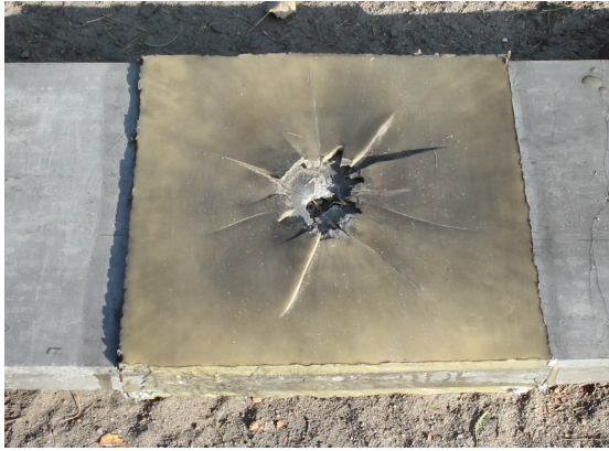
FIGURE 8. The effect of an explosion on an HPFRC panel with PU coating on both sides; impact side.
