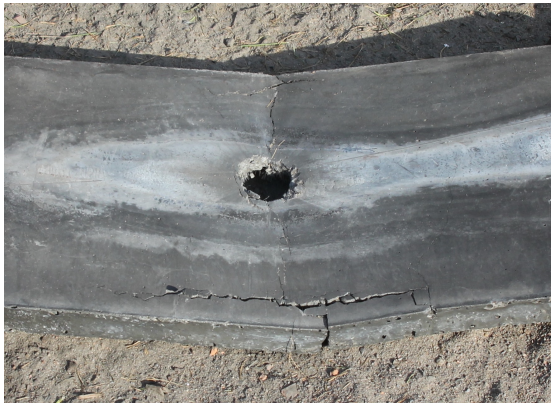
FIGURE 12. Complete failure of a bare HPFRC panel due to blast; impact side.
