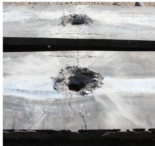
FIGURE 7. The effect of an explosion on an HPFRC panel without PU coating; rear side.
