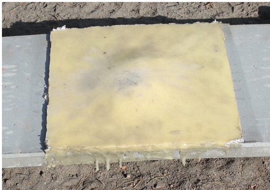
FIGURE 9. The effect of an explosion on an HPFRC panel with PU coating on both sides; rear side.
