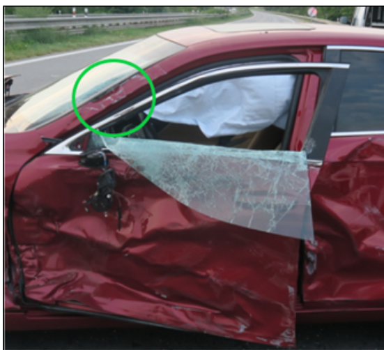
(B). Damage to the red vehicle on the left rearview mirror.
