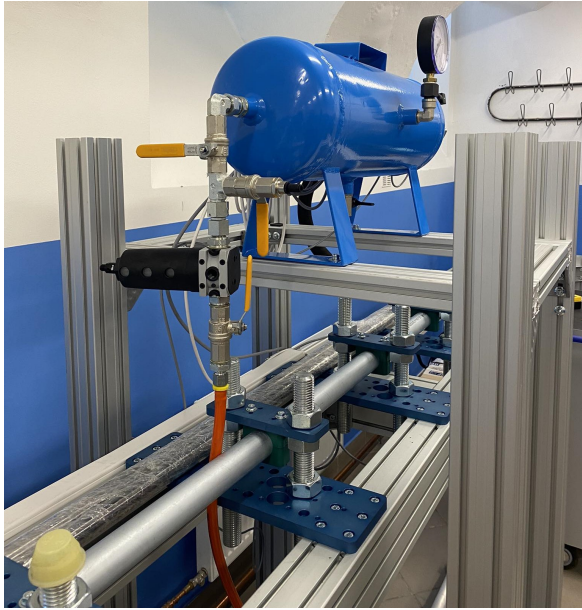
FIGURE 4. The pneumatic launch system.
