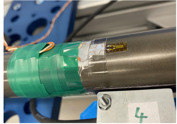
FIGURE 5. Strain gauge mounted on the bar's surface.
