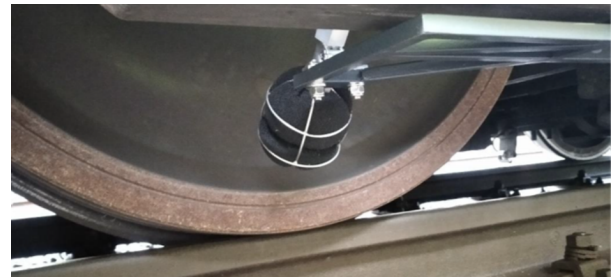
FIGURE 2. Position of the microphone for measuring the contact noise between the rail wheel and the rail on the MVŽSv2 diagnostic vehicle [12].
