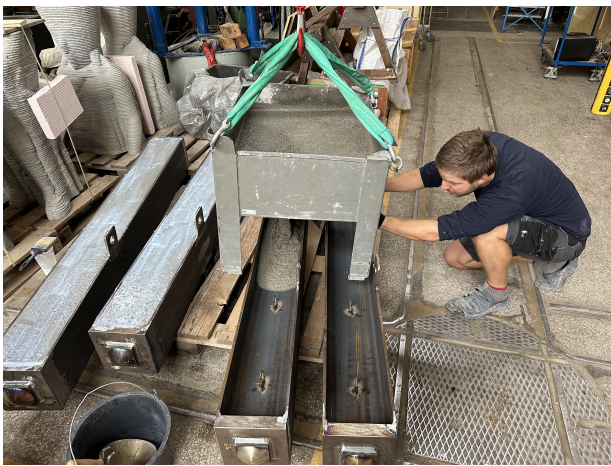
FIGURE 4. Process of casting of the test specimens.
