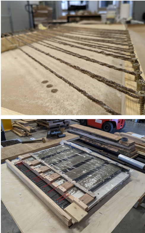
FIGURE 1. Homogenised hybrid rovings from AR glass and flax with epoxy resin and sprinkled with sand (top) and concreted samples in a framework (bottom).
