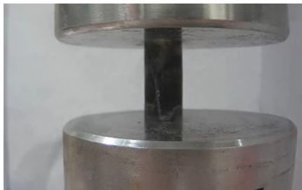
FIGURE 4. First crack, time 170 s.
