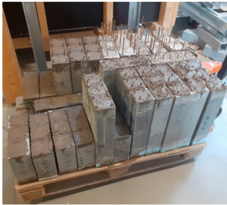
FIGURE 3. Hollow HPC skin during the process of hardening before cutting (on the top) and specimens already cut and filled with RAC after the process of concreting with visible steel reinforcement in the corner (on the bottom).
