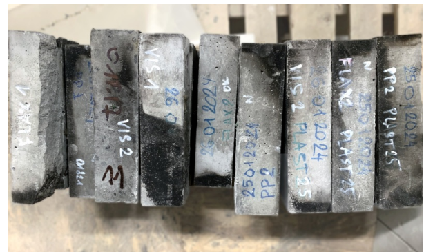
FIGURE 5. Samples after the fire experiment.
