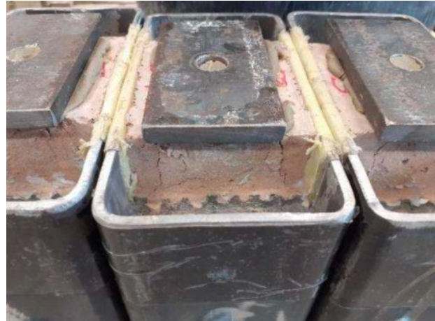
FIGURE 3. Steel-cased samples after testing.
