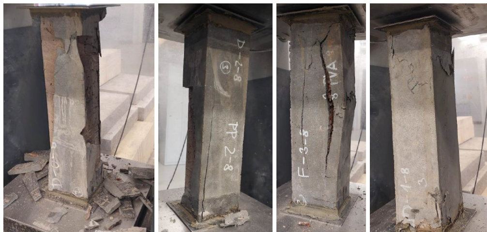
FIGURE 3. 8 mm shells filled with RAC by materials from left: plain concrete, PP FRC, PVA FRC, TRC (carbon grid).
