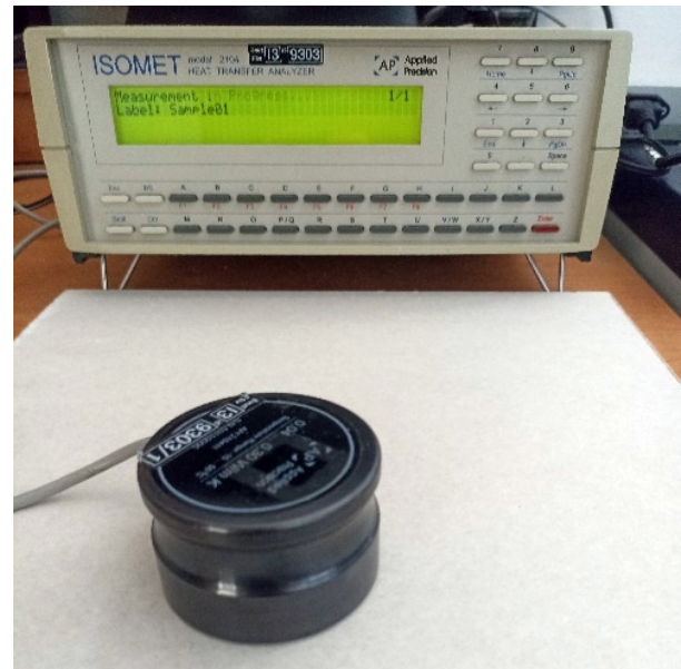
FIGURE 4. Measurement of thermal properties using the ISOMET 2104.
