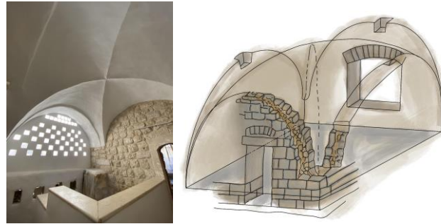
Figure 7: Represents the plan and section of the layers used in the process of establishing the vault in a traditional dwelling. (Drawing by Author 2023)
