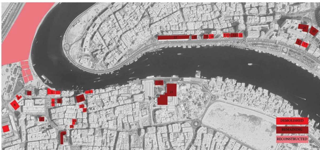
Figure 9: Comparative Diagram of several Demolished and Remaining Modernist Buildings overlaid on a satellite image. Base Image captured from Google Maps.
