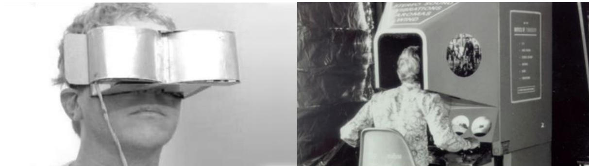
Left, Figure 2-1: The Telesphere Mask , invented by Morton Heilig in 1960. Right, Figure 2-2: The Sensorama , built in 1962, was an immersive device designed to simulate a bike ride. (Scheinerman, 2009)
