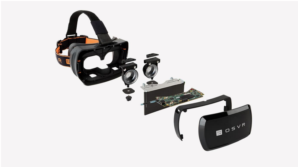
Figure 1: Illustration of the internal components of the augmented reality headset. (Barrial, 2015)
