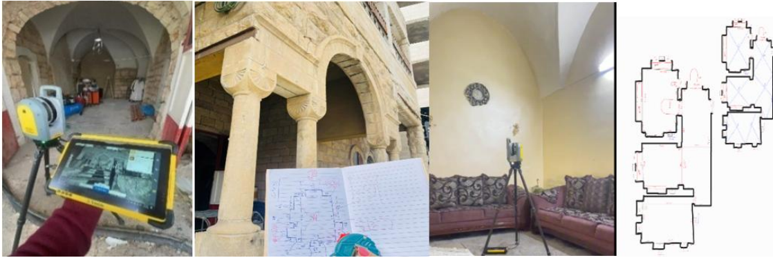
Figure 6 represents the stages of taking measurements, documenting, and drawing plans of the Zaroo House. (Author, 2024)
