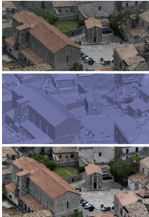
Figure 1 Gerace (RC), three churches square. Axonometric view of the point cloud (top), of the TIN mesh (center), of the textured mesh (bottom) (Graphic elaboration by Lorella Pizzonia).
