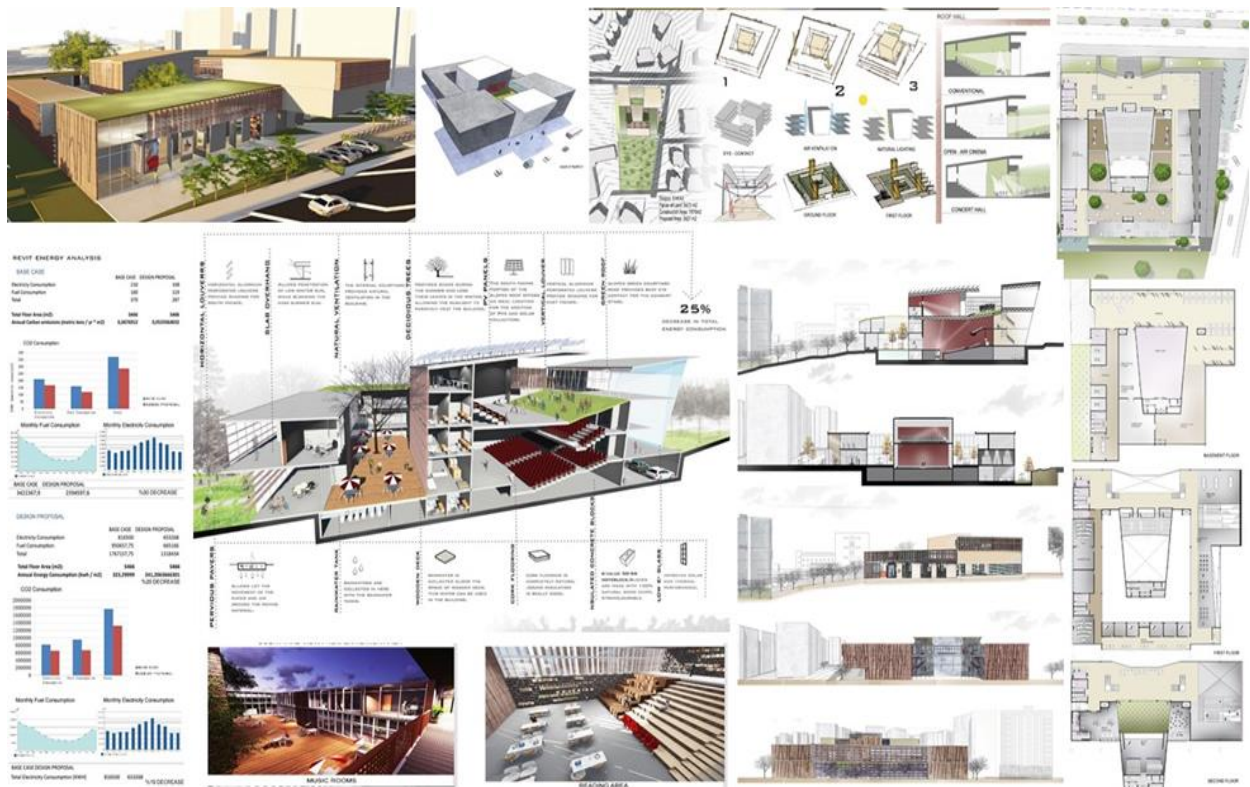
Figure 2. Bornova culture center by “Ezgi Çam” was exploit the idea of a center mass that included the major program spaces while it was surrounded by lower mass that included other spaces. This strategy provided good quality of natural light and natural ventilation throughout the open space created between the two masses as well as various open and semi open spaces. Furthermore, the orientation, height, and size of masses considered the natural resources such as wind, natural light, rainwater, etc. as well as the choice of sustainable materials and various shading elements. The design expected to save 25% in annual energy consumption and 30% in CO 2 emission. The project collected 19 points of the total 19 points of the sustainability checklist elements.
