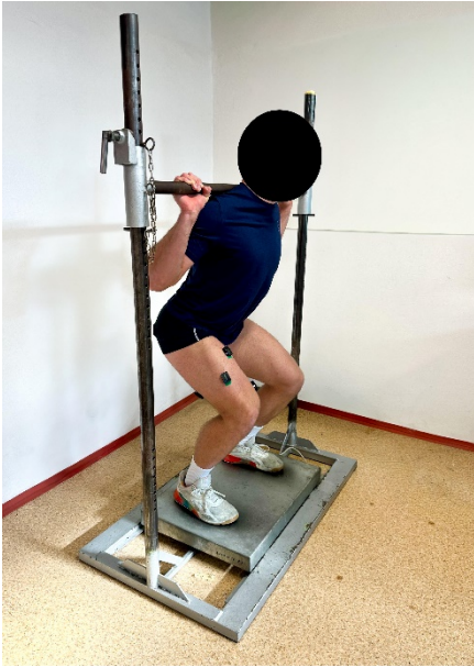
Figure 1 Peak force and surface electromyographic (EMG) activity during maximal isometric high-bar back squat at 90° knee flexion
