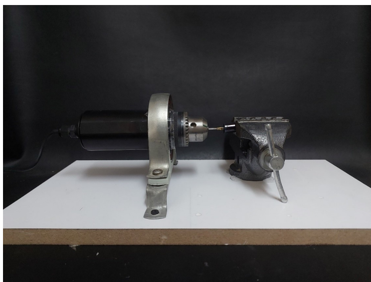
Figure 2. Custom-made device for measuring torque and reverse torque.
