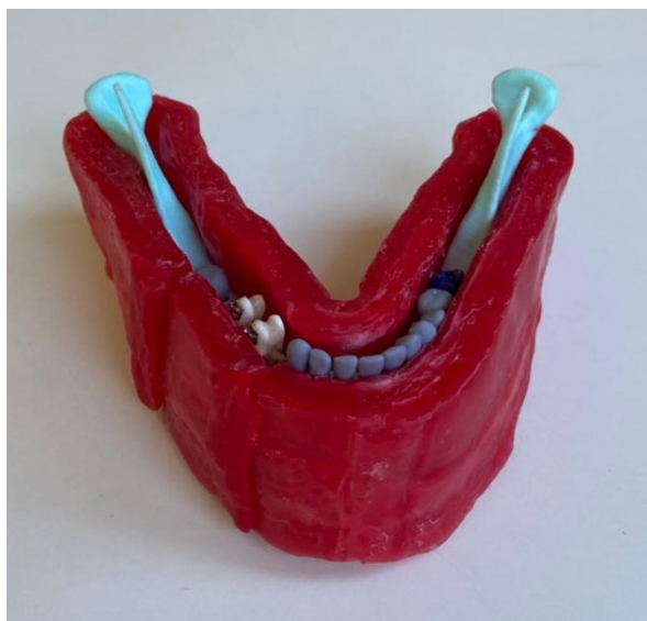
Figure 1. Bovine rib with extracted human premolars adapted to a 3D printed jaw surrounded by a 15 mm layer of wax 7
