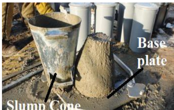
Fig.1- Slump Flow Test
