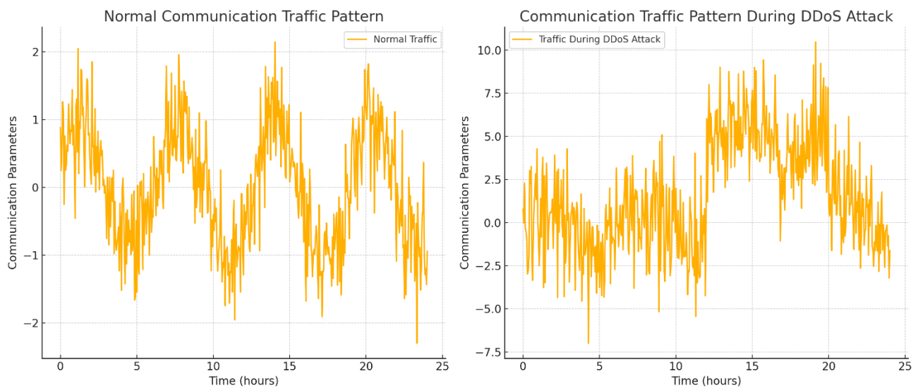
Fig. 3 : Graphical results showing the normal communication traffic patterns & during the DDoS attacks
