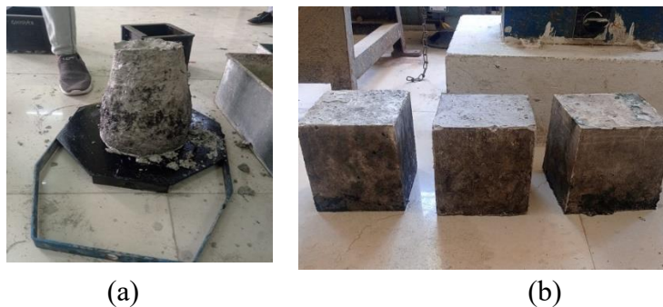
Fig. 5 Images showing (a) Slump cone test for SGC prepared with SS/GGBS = 0.35 and (b) SGC demolded cubes after 24 hours
