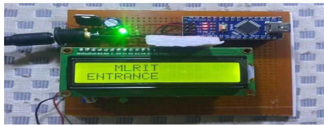
Fig-4 (a): Display of LiFi receiver at pole-1
