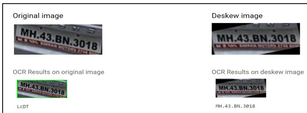
Figure 7: OCR Result on cropped number plate image (before and after deskewing)
