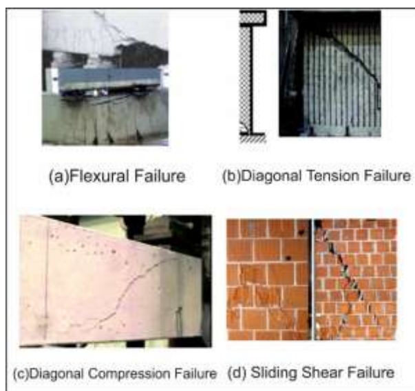
Figure 1 Three Cases of Shear Failure
