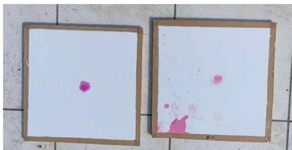
Figure 14. Application of Rhodamine dye on wall putty specimen
