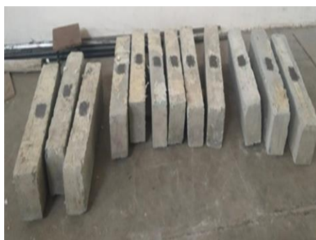
Figure 3 Reinforced concrete beams after 28days curing
