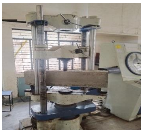
Figure 4 Testing arrangement of RC beam specimen.
