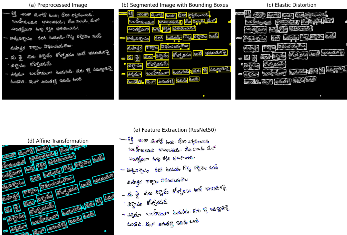
Figure 4. (a) Preprocessed Image (b) Segmented Image with Bounding Boxes (c) Elastic Distortion (d) Affine Transformation (Data Augmentation functions) (e) Feature Extraction
