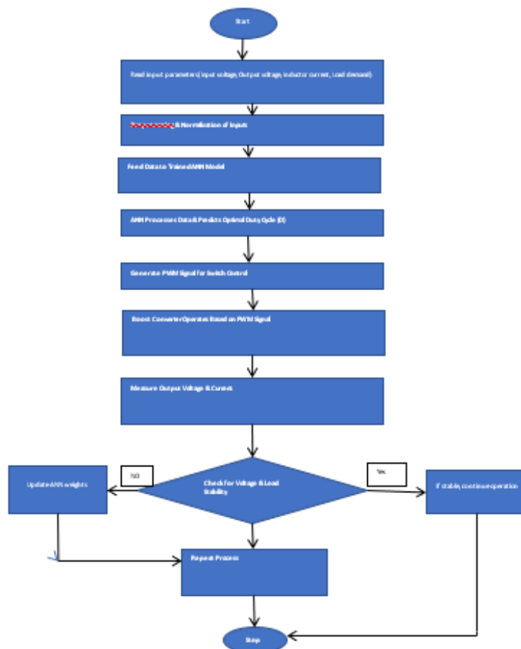
Fig-2 Flowchart for PV Supplied SL-SC Based High Voltage Gain Artificial Neural Networks controlled Boost Converter for HV EV Charging System
