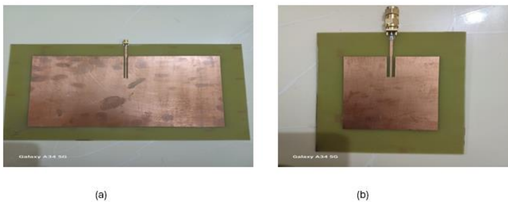
Figure 7: Hardware implementation of a) F1 Microstrip antenna for 433 MHz, b) mF1 Microstrip antenna for 866 MHz
