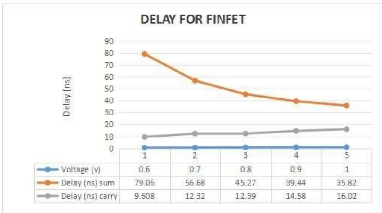
Figure 4: Sum and Carry Delay Trends in FinFET Adder Design
