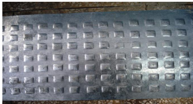
Fig. 2: Photographic view of absorber plate roughened by formation of square protrusions.
