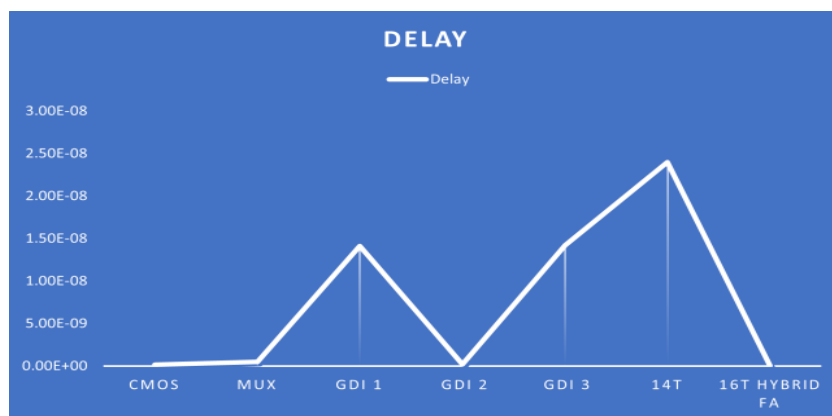
Fig.11. Comparison of Delay Analysis of adders
