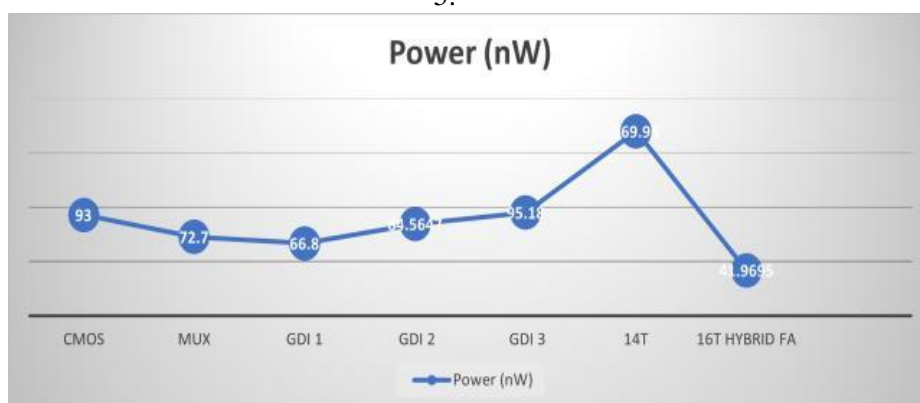
Fig.10. Comparison of Power consumption of adders
