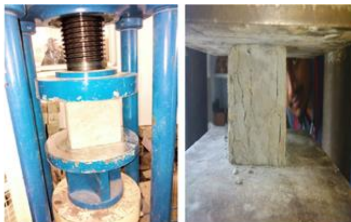
Figure 4.1 & 4.2 Compressive strength testing specimen in concrete & Concrete cube specimen after testing
