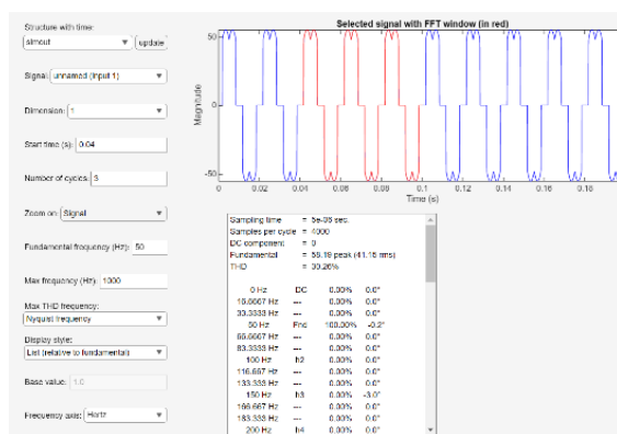
Fig. 4 FFT analysis at different frequency with 30.26% of THD
