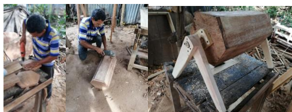
Figure 1: Construction of hexagonal rotary fermenter
