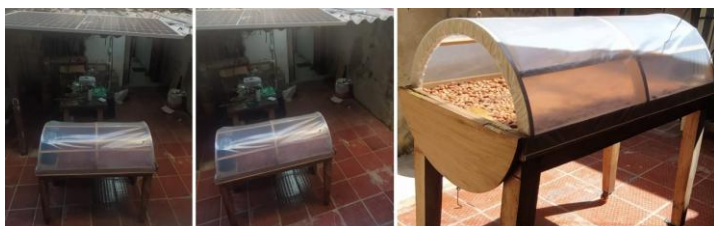
Figure 4: Designed greenhouse dryer connected to a solar panel and two electrical fans.
