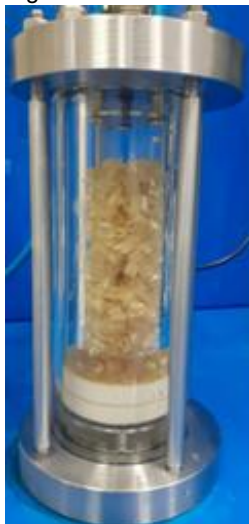
Figure 2: Bed containing hydrogel Raschig rings ( W = 0.80 g water/g hydrogel) for water removal from fuels
