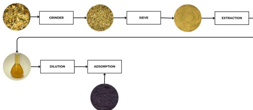
Figure 1: Steps in the yerba mate preparation, phenolic compounds extraction and adsorption
