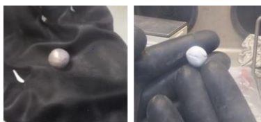
Figure 9: Comparison of a pure sodium ball (on left) with an oxidised ball
