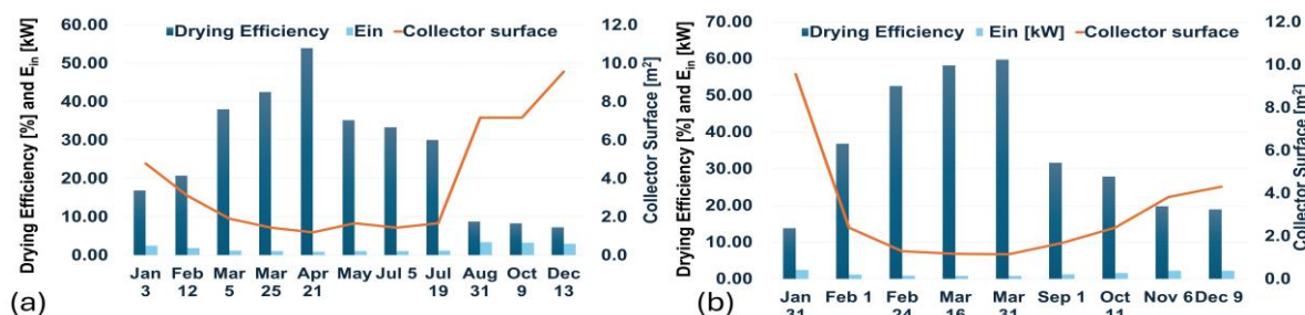
Figure 3: Apple drying efficiency for each test and amount of energy incident on the dehydrator. (a) Tests from 2023, (b) Tests from 2024
