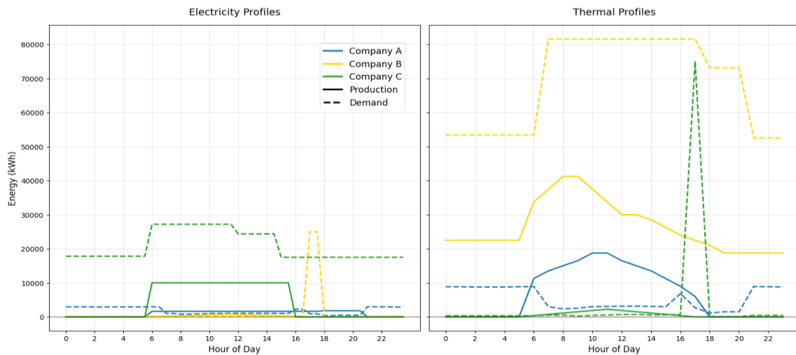
Figure 3: Demand and production profiles for electricity and thermal energy of the companies
