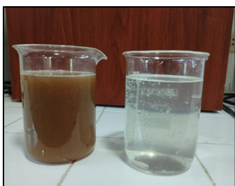
Figure 4: Agricultural coffee wastewater before and after electrocoagulation treatment
