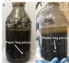
Figure 1: Digestate samples at the end of anaerobic digestion, containing fragments of paper and plastic collection bags. (a) Reaction mixture with Paper bag 1 (PaB1); (b) Reaction mixture with Plastic bag 2 (PiB2)
