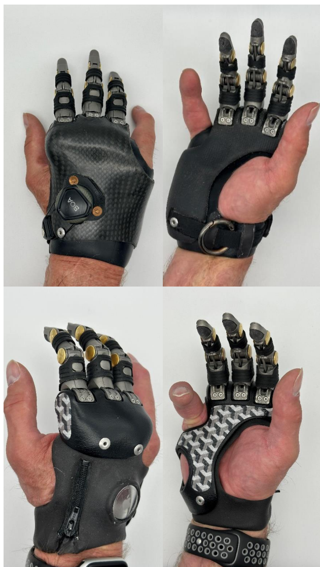
Figure 1: Top row showing dorsal and palmar views of Jeff's carbon fiber laminated prosthesis. Bottom row showing dorsal and palmar views of Jeff's additively manufactured prosthesis. The significant difference in bulk and rigid areas between the two prostheses is clearly seen.
