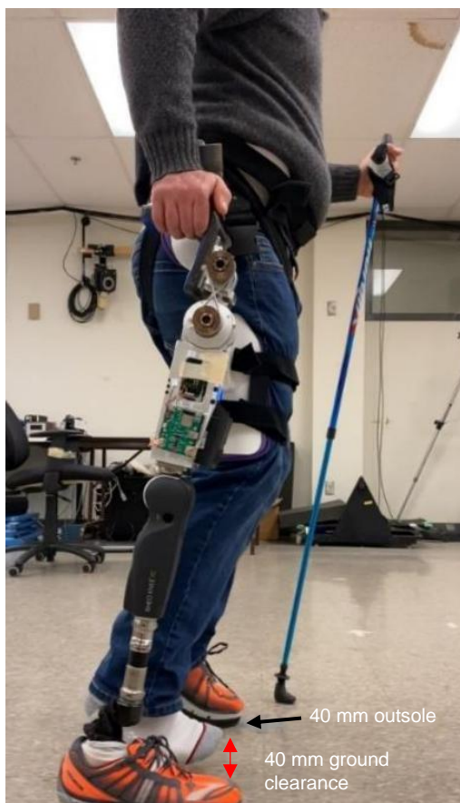
Figure 7: Hip disarticulation simulator 23 setup with PHP, Össur Rheo 3 knee joint, and Össur Pro-Flex XC foot. Participants wore an elevated outsole on the intact limb to create 40 mm ground clearance for the right foot during stance.
