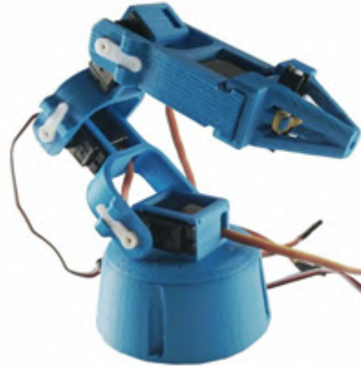
Figure 8: 3D printed robot arm based on Arduino robotic platform.
