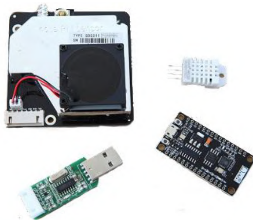
Fig. 3. The main components of the prototype for Luftdaten
