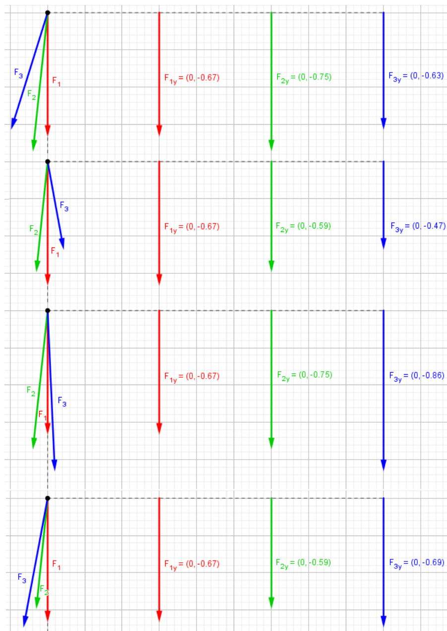
Figure 14: Dynamic vector diagram of Y-component F_y of the resultant forces acting on the projectile in four cases (from top to right): t_i = 0, rot = 1 ; t_i = TM, rot = 1 ; t_i = 0, rot = -1 ; t_i = TM, rot = -1 .
